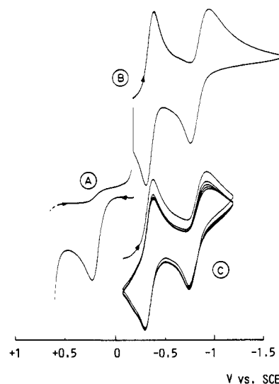
Figure 3. Cyclic voltammograms of complex 2 in DMF/0.1 M tetrabutylammonium perchlorate: (A) oxidation scan; (B) reduction scan; (C) reduction scan, some cycling at 100 mV/s.
